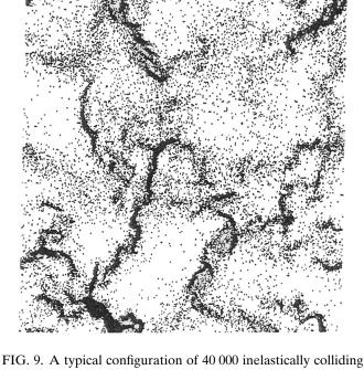
FIG. 9. A typical configuration of 40 000 inelastically colliding particles, exhibiting clustering in two dimensions. Here the coefficient of restitution is 0.6, the time corresponds to 500 collisions per particle, and the average area fraction occupied by particles is 0.05. The system is started with a spatially uniform distribution of initial velocities and allowed to evolve without further energy input, after Goldhirsch and Zanetti (1993).
