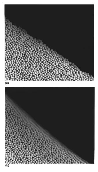
FIG. 1. (a) A pile of mustard seeds that is tilted to an angle lower than the angle of repose. (b) The same pile after the slope has been increased slightly to create an avalanche. Note that the flow occurs only along the surface and that the seeds deeper within the pile do not participate in the motion.
